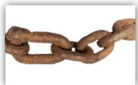
Incorrect Hardware & Pitting
