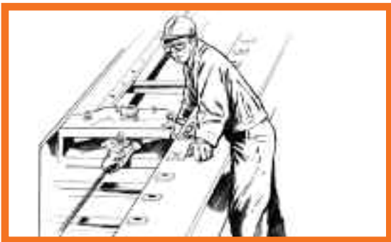
Observing a pull test from this position may result in serious injury or death !
