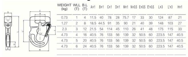
Ultimate load is 4 times the Working Load Limit.
