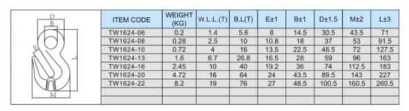
Ultimate load is 4 times the Working Load Limit.
